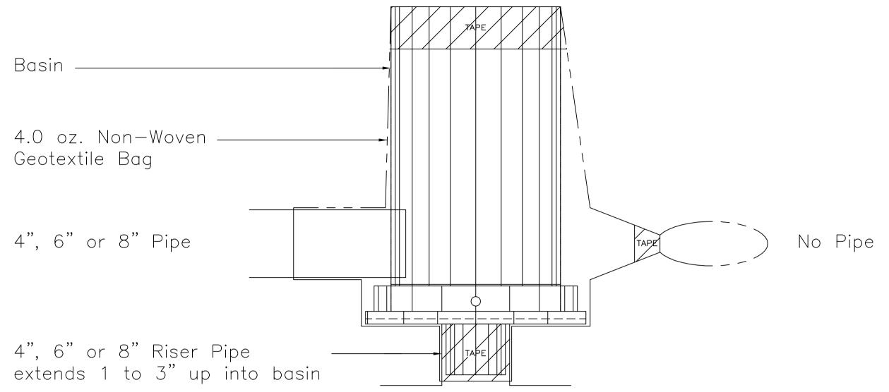
6. Sod around the basin. If sod work is not done immediately after the installation of the basin, a 15 inch square piece of a geotextile fabric should be placed on the top frame and held in place by the placement of the grate on the frame until the
