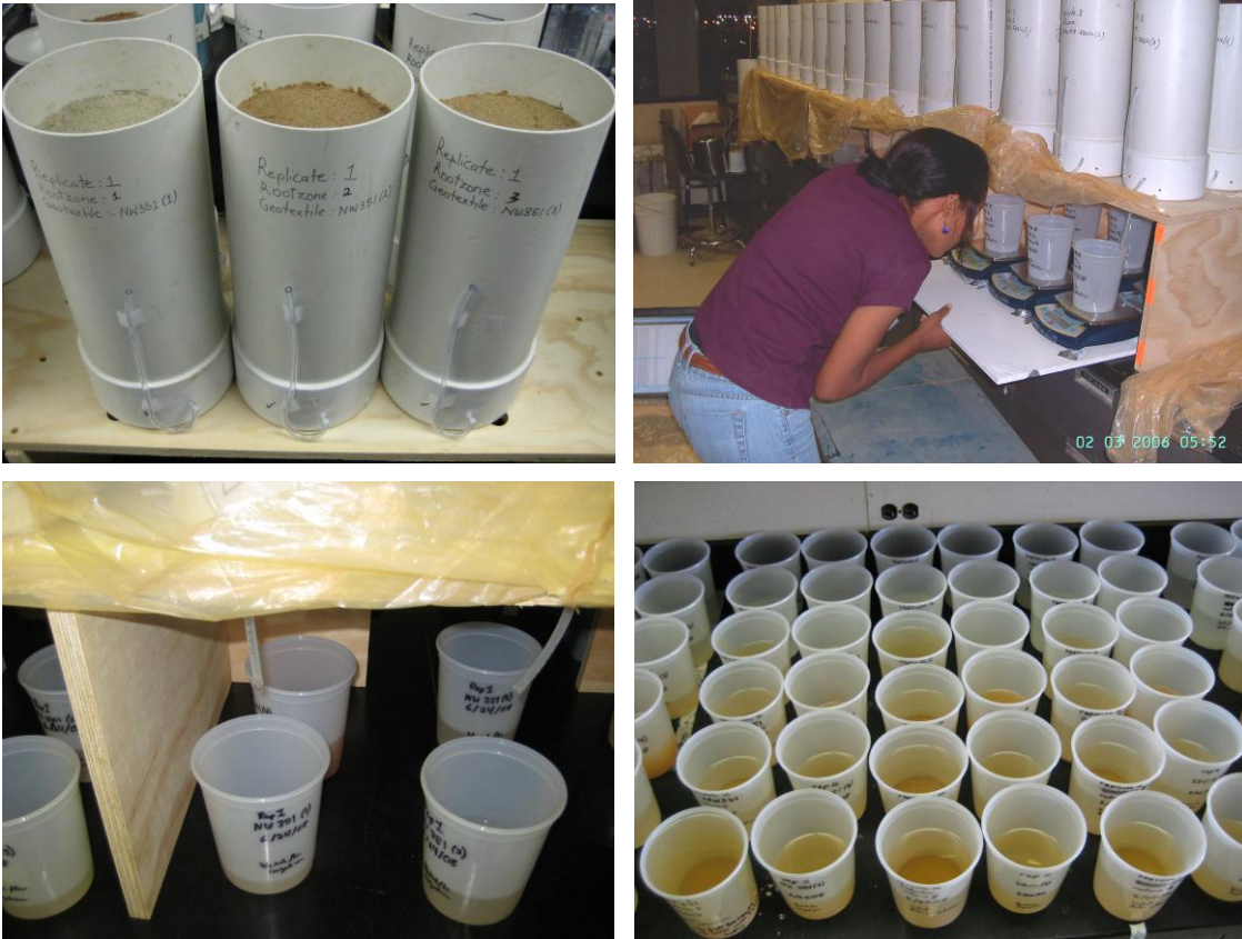
Figure 22. Columns used to test for clogging of geotextile pores (upper left), monitoring drainage rates (upper right), collection cups for drainage water (lower left), and cups used to flocculate particles passing through the columns (lower right).
