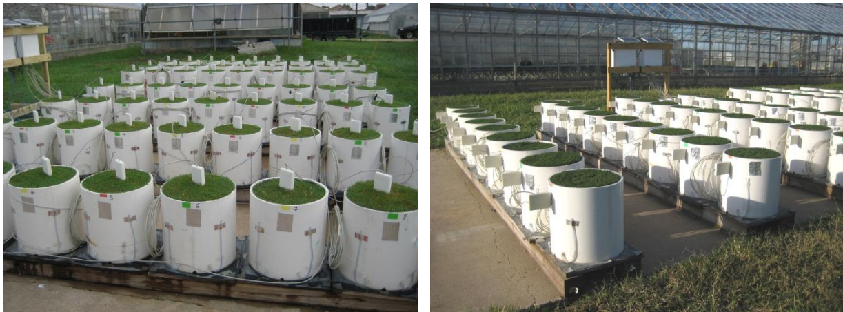
Figure 4. TDR probes installed vertically (left) and horizontally (right) at 3-in (75 mm) depth in the test greens. Vertically installed TDR probes measured average profile water content and horizontally installed probes measure average water content at the depth of installation.
