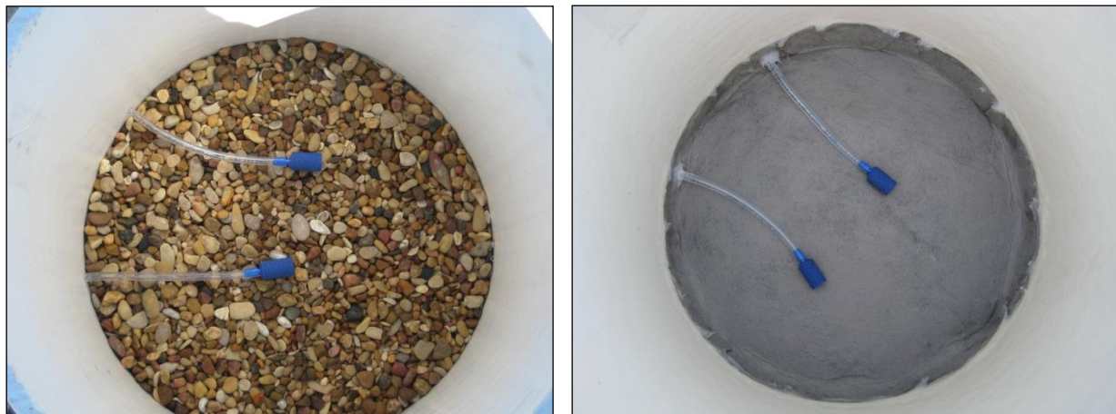
Figure 3. Tensiometer-manometers above gravel (left) and geotextile/AirDrain (right) drainage layers at the bottom of the test greens before root zone mixtures were added.
