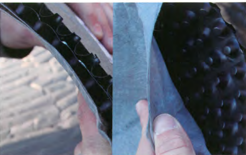
Over 11 miles of the waffle drain pipe was installed throughout Westmoreland Country Club. The two pieces of plastic are wrapped by a geotextile fabric.
